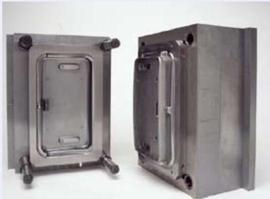
Theka Formverktyg AB produced this plastic mould tool for vehicle number plates using Toolox 33 for the core and Toolox 44 for the cavity. The high stability and ease of machining was particularly noted.
