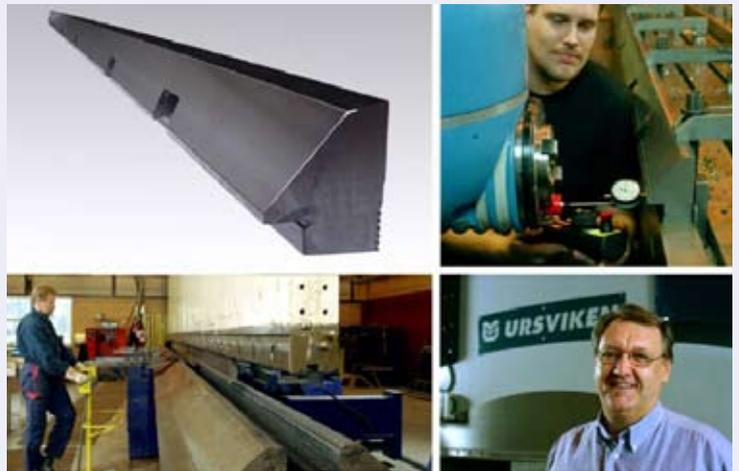
Ursviken Pullmax produced this 3 metre long press-brake blade in Toolox 33 and measured only 0,7mm maximum deflection from end to end. Milling speed was also 25% faster than with the previous material 1.2312 (P20 with Sulphur). This demonstrates both the superb stability of Toolox 33 and its free-cutting qualities.
